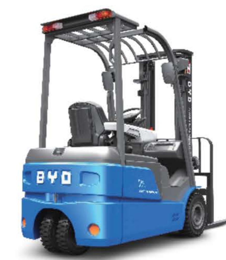
ECB16 Load capacity: 1.6 ton Curb weight: 3,100 kg Min. turning radius: 1,570 mm Voltage: 80 V Battery capacity: 270 Ah
