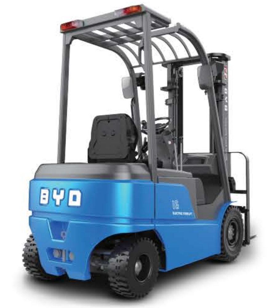
ECB18 Load capacity: 1.8 ton Curb weight: 3,300 kg Min. turning radius: 1,640 mm Voltage: 80 V Battery capacity: 270 Ah
