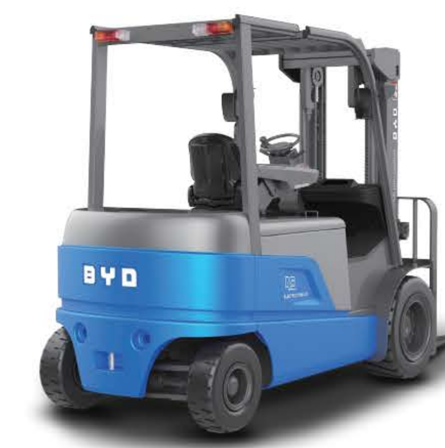
ECB45 Load capacity: 4.5 ton Curb weight: 7,030 kg Min. turning radius: 2,600 mm Voltage: 80 V Battery capacity: 540Ah/810Ah
